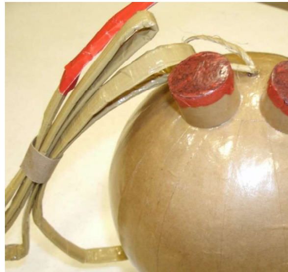
Fig. 2.16: Visco green fuse leader (left) and thin black match leader (right). Fig. 2.17: Shell leader with red safety cap attached to 6-inch ball shell. Photos: IPM Universal
