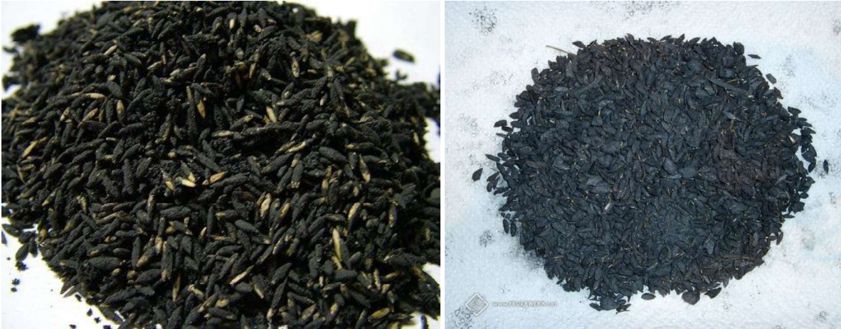
Fig. 2.35-2.36: Example of rice hull powder. Black Powder coated rice hulls. Photo: PyroFlo, Feuerwerk.net
