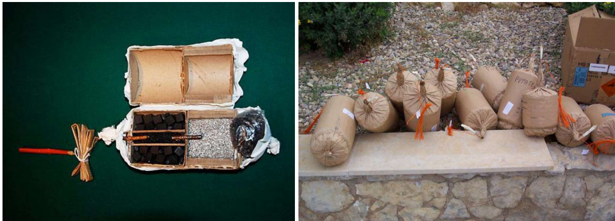
Fig 2.06: Examples of cylindrical shells and cut-away. Photo: by dagabu from AmateurPyro.com forum. Fig. 2.07: Here is a typical Maltese-style Italian (200mm) cylinder shell. Photo: Martarello Group, Italy
