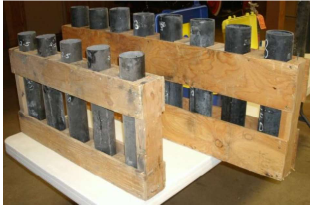
Fig. 2.11: Wooden racks holding 2.5-inch and 3-inch HDPE mortar tubes for aerial shells. Photo: IPM
