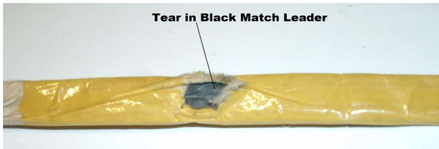
Fig. 3.35: Tear in quick fuse match. Photo: IPM
