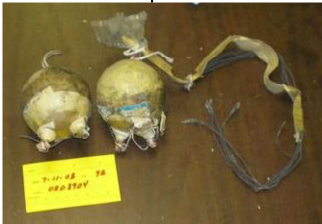
Fig. 3.20: Dud 3-inch ball shaped aerial shells. Photo: courtesy of Twin Falls Police Bomb Squad. Fig. 3.21: Dud shells that have been water damaged and without lift charge. Photos: IPM
