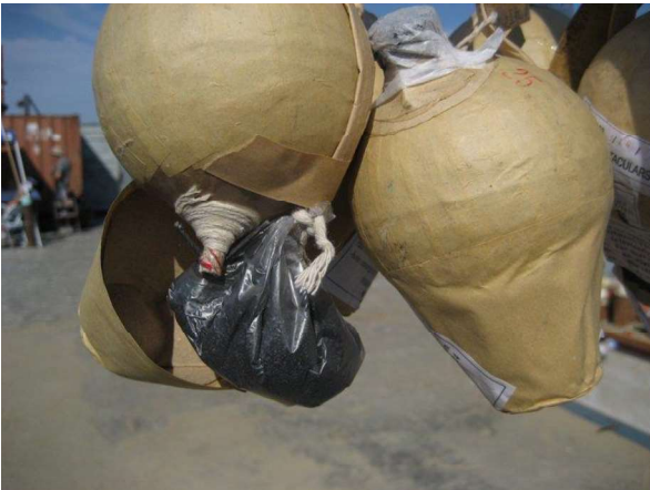
Fig. 3.01: Shell lift charge bags; photo Pyro Spectaculars. Fig. 3.02: Black powder lift charge broken. Photo: Skylighter.com
