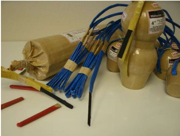
Fig. 3.39: Black match leaders with red safety caps. Photo: IPM
