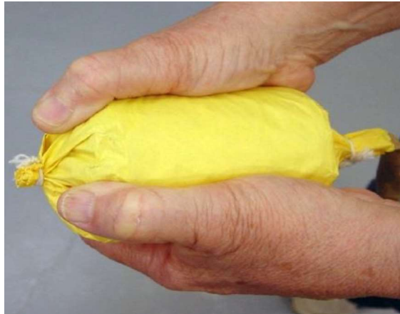
Fig. 3.30: Powder lift on bottom of aerial shells. Photo: Northern Lights Pyrotechnics
