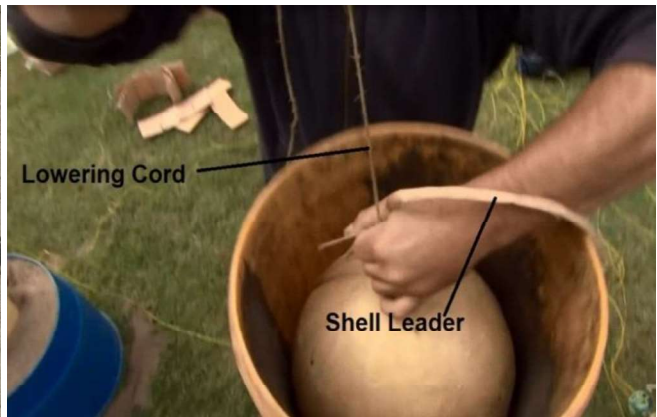
Fig. 3.41-3.42: Lowering cord on larger aerial shell. Green lowering rope on large shells. Northern Lights Pyro
