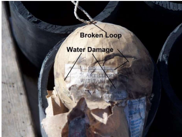
Fig. 3.43: Water damaged shell. Photo: IPM. Fig. 3.44: Damaged shell with dent. Photo: Journal of Pyrotechnics
