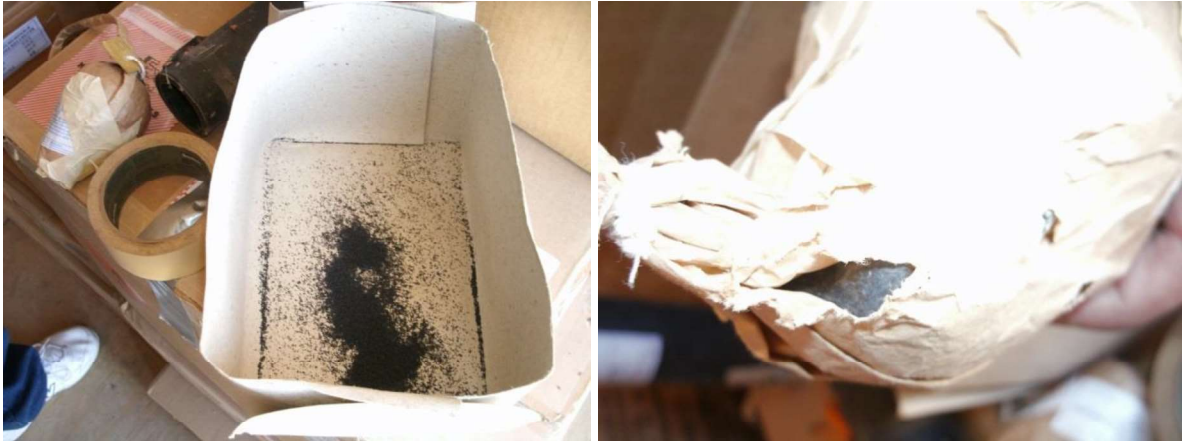
Fig. 3.28: Lift powder seen on bottom of shell box. Fig. 3.29: Tear in the bottom of lift powder. Photos: IPM
