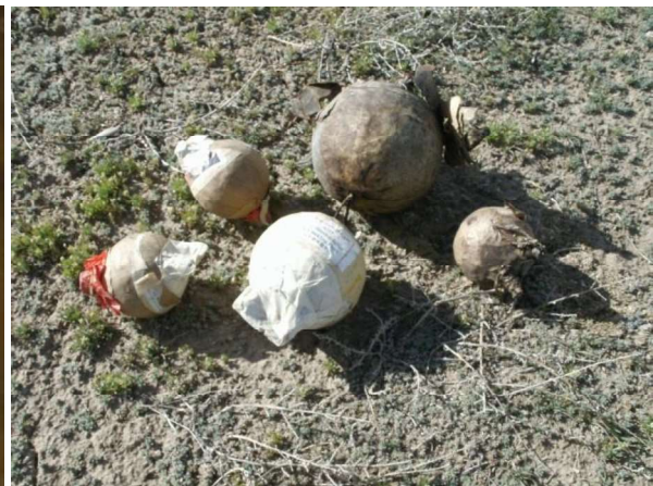
Fig. 3.20: Dud 3-inch ball shaped aerial shells. Photo: courtesy of Twin Falls Police Bomb Squad. Fig. 3.21: Dud shells that have been water damaged and without lift charge. Photos: IPM
