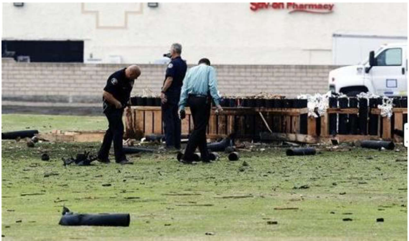
Fig. 3.13: Simi Valley explosion site where HDPE mortars are displaced due to double-break shell malfunction “detonation”. Photo: Nick Ut, AP
