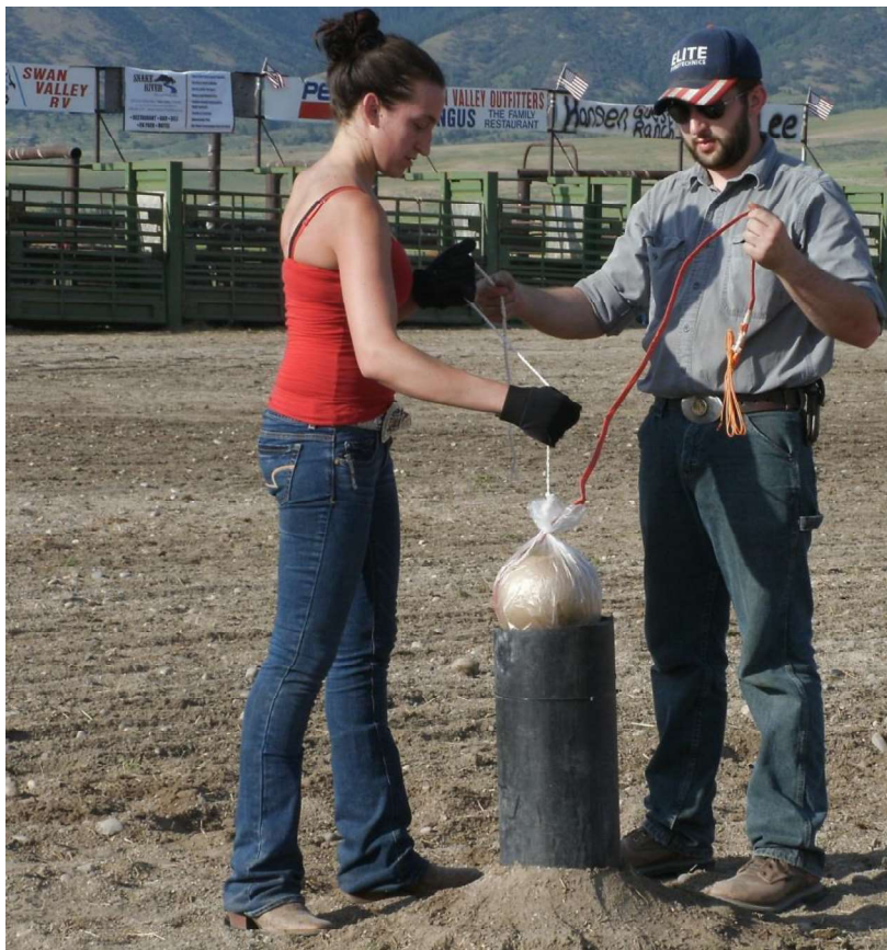
Fig. 3.45-3.47: Technicians Rainey, Kevin Josephson and T.J Williams carefully loading 8" shells with the help of lowering cord. Photo credits: Northern Lights Pyrotechnics & IPM Universal
