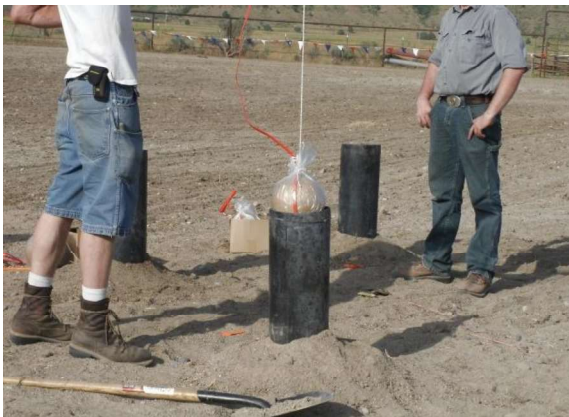
Fig. 3.41-3.42: Lowering cord on larger aerial shell. Green lowering rope on large shells. Northern Lights Pyro
