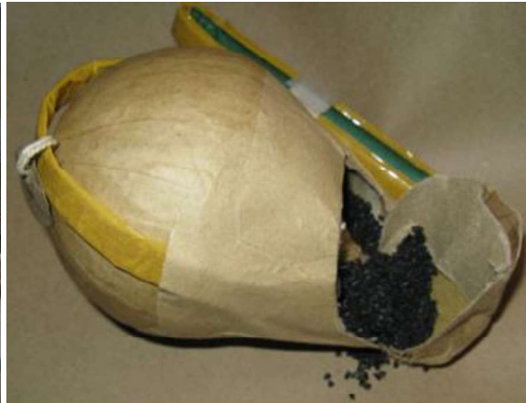
Fig. 3.01: Shell lift charge bags; photo Pyro Spectaculars. Fig. 3.02: Black powder lift charge broken. Photo: Skylighter.com
