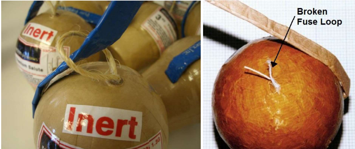
Fig. 3.33: Leader attached by a fuse loop which is intact (left) Photo: IPM. Fig. 3.34: (right) broken loop, JPyro
