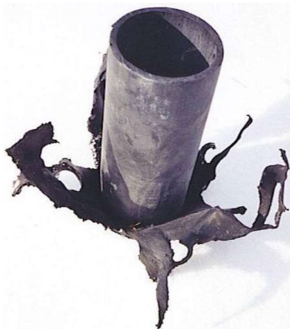
Fig. 3.12: Large mortar shredded by a shell “detonation”. Photo: IPM.
