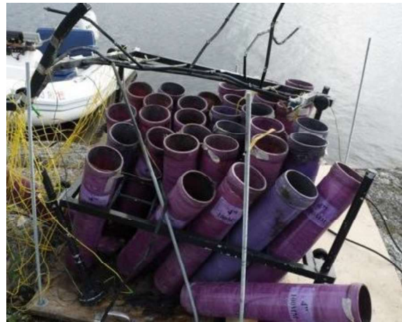
Fig. 3.27: Mortar rack test after shell detonation. Photo: Fireworks FX, Inc. Canada
