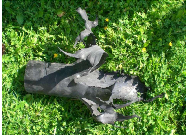
Fig. 3.11: Blown 3-inch mortar. Photo: user Raini at Feuerwerk.net Wiki
